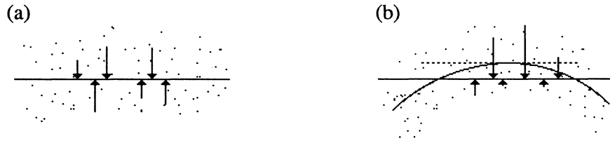
FIG. 5. Consider a noisy one-dimensional set. In the absence of curvature (a), the mean of the corrections is zero. If the underlying manifold is curved (b), projection onto the fitted straight line yields a nonzero mean correction, which can be subtracted to come closer to the desired tangent.
